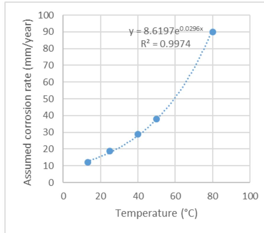
Adjustments due to low flow velocities and high time during some corrosion rate tests (loop); Equation extrapolated to temperatures lower than 13°C.
