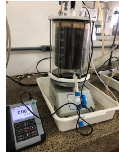
A: first day of experiment, **with only CO<sub>2</sub> and N<sub>2</sub> in the gas mixture. Before heavy precipitation of iron carbonate.**
